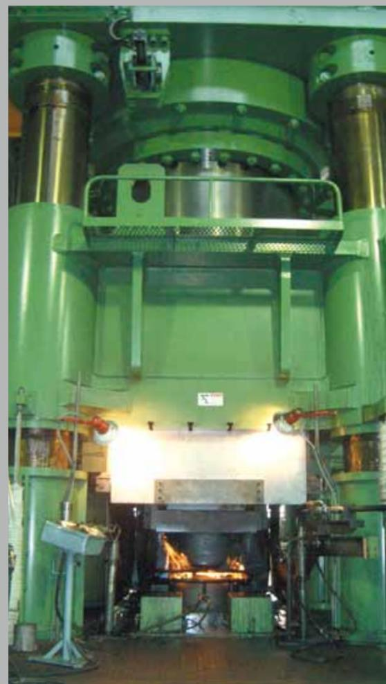
Our 9,000 tonne hydraulic forging press
