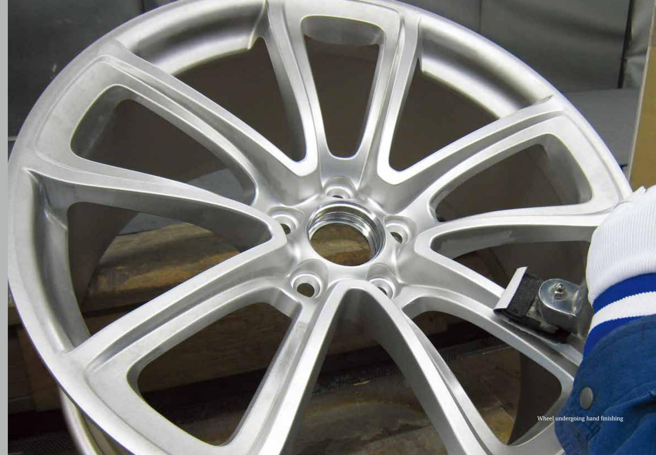
Wheel undergoing hand finishing
