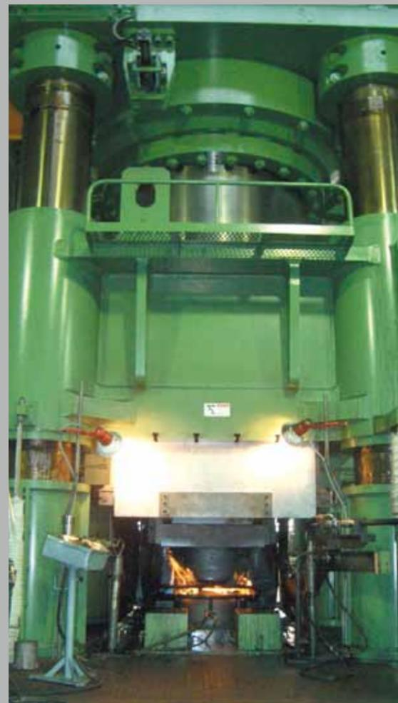
Our 9,000 tonne hydraulic forging press
