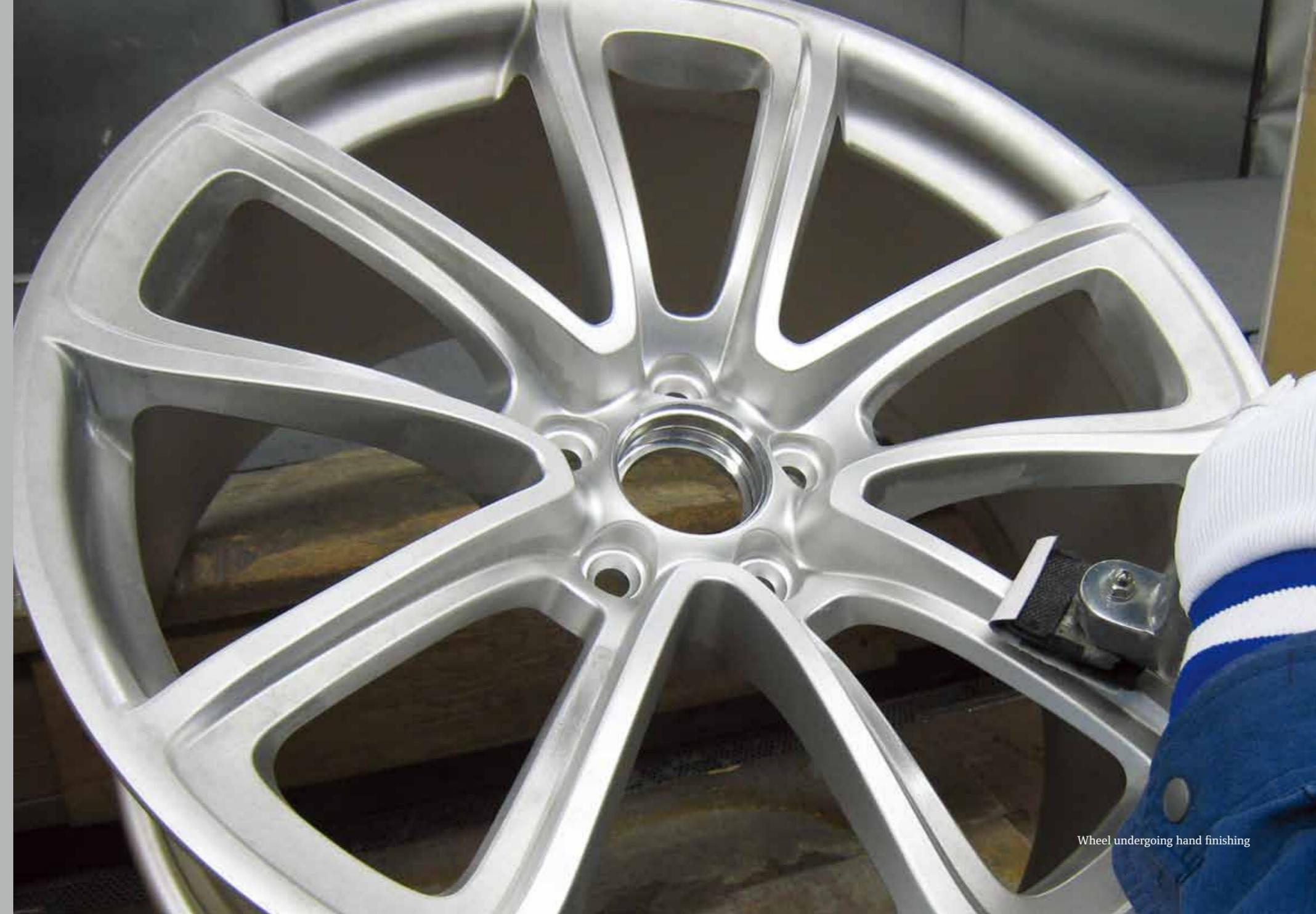
Wheel undergoing hand finishing
