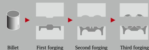
Washi Beam have developed a safe and consistent way to forge with pressures of more than 4 tonnes per square centimetre – approximately 57,000lbs per square inch.
